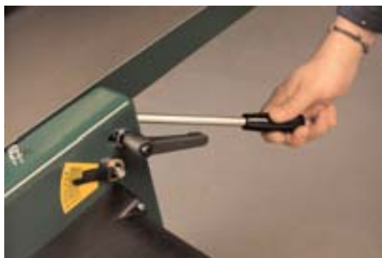
To adjust cutting depth when surface planing you slacken off a Bristol lever and move a steel lever up or down
