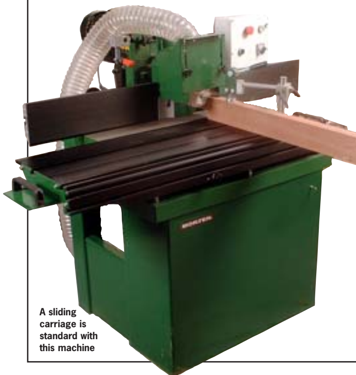
Graduated handwheels provide fine adjustment for fences, rise and fall, lateral movement and so on
