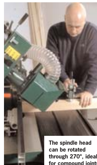
You can move the spindle head accurately across the table. This is superb for jobs such as deep tenons
