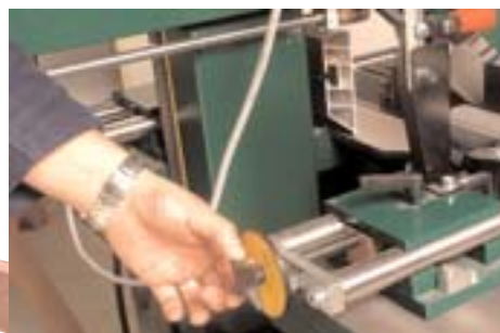
Graduated handwheels provide fine adjustment for fences, rise and fall, lateral movement and so on
