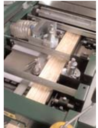
There are viewing windows in the top so you can see timber as it passes through (here cover is removed)
