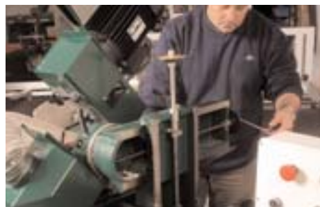
Graduated handwheels provide fine adjustment for fences, rise and fall, lateral movement and so on
