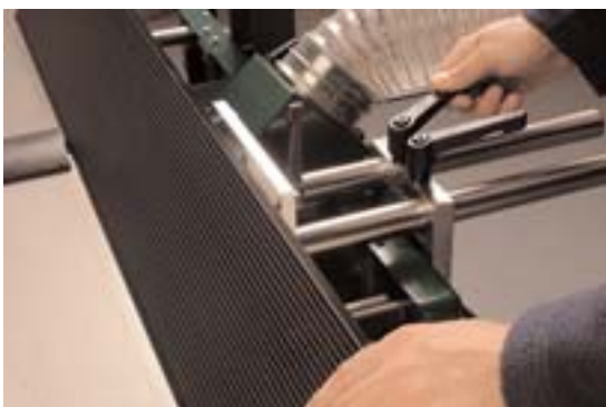
Twin Bristol levers lock the aluminium fence on hefty steel rods and castings. It can be locked up to 45° and calibrated
